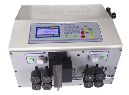
WPM Series Full-automatic Computer Wire Stripping Machine made by our factory is suitable for cutting, head-stripping, tail-stripping and middle-stripping of single –strand, multi-strand and sheathed wire. The maximum processing cross-sectional area is 0.1-70mm 2; the maximum cutting length is 100m, head-stripping 200mm and tail-stripping100mm.
