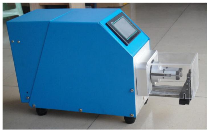
Brief Description: mainly used for a single line, coaxial cable, and special processing, using the most advanced rotary tool carrier, improve the processing accuracy and speed. Use of a specific axis positioning device and the rotary cutter way, up to nine-stripping blades can be replaced without the corresponding processing of various sizes and skin wires.
